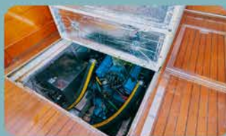
Twin 350 Jasper Engines & Paragon Transmissions
